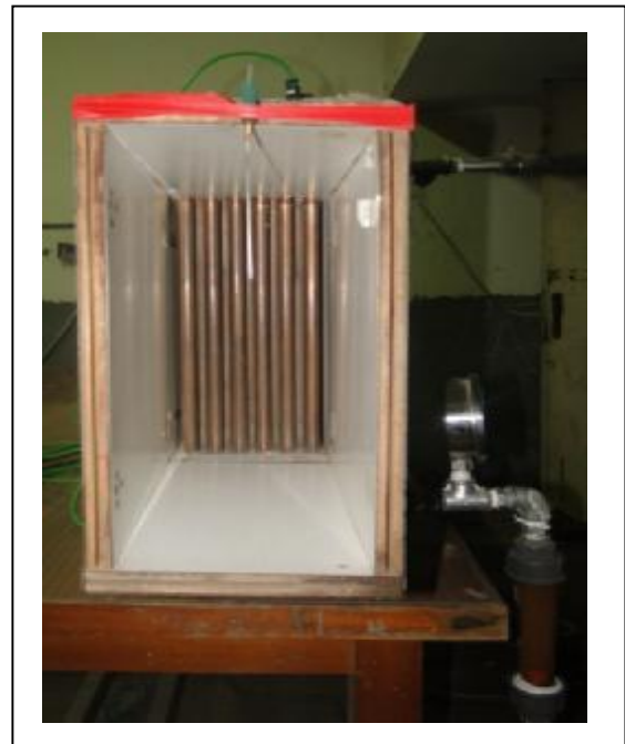
Fig. 6. Plain Tube Heat Exchanger.
